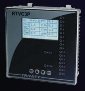
The RTVC3P controls the automatic system for correction of the power factor. It is a KVAR based controller which controls up to 16 capacitor banks optimally to achieve near unity power factor and also measures/calculates various electrical parameters. RTVC3P is meant for use in three phase four wire electrical systems. The main features of the RTVC3P are:
