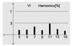
The fourteenth, sixteenth and eighteenth pages show the histogram of up to 15<sup>th</sup> Odd Harmonics in percentage form of R-phase, Y-phase and B-phase volatge respectively.
