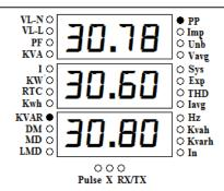
The 6<sup>th</sup> page shows Phase wise KVAR for R, Y and B phase. This page indicated by "**KVAR**" and "**PP**" LEDs glow. This Page will be not available in the 1P2W installation.
