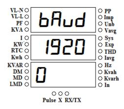
2. Press key again. Immediately 'P' starts blinking which shows that the parameter can now be changed. Select the Baud rate by pressing and keys according to your desire and then press key to save the parameter.
