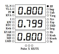
The 4<sup>th</sup> page shows Phase wise PF for R, Y and B phase. In case of leading PF, the unit will show "-" sign for all three individual phases. This page indicated by "**PF**" and "**PP**" LED glow. This Page will be not available in the 3P3W and 1P2W installation.
