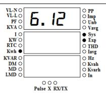
The 11<sup>th</sup> page shows System Export KWh. This page indicated by "**Kwh**", "**Sys**" and "**Exp**" LED glow.
