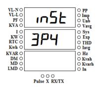
2. Press key again. Immediately 'P' starts blinking which shows that the parameter can now be changed. Select the installation type by pressing and
