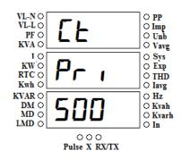
2. Press key again. Immediately 'P' starts blinking which shows that the parameter can now be changed. Set the CT PRIMARY by pressing and
