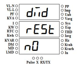
2. Press <sup>(ROB)</sup>/<sub>(NIR)</sub> key again. Immediately 'P' starts blinking which shows that the parameter can now be changed. Select "JE5" by pressing ▲ and ▼ keys and then press <sup>(ROB)</sup>/<sub>(NIR)</sub> key for resetting Demand Data and after the <sup>(ROB)</sup>/<sub>(NIR)</sub> Key Press unit automatic reset.
