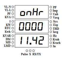
The 37<sup>th</sup> page shows ON Hour. This page indicated by "**Dn**H**r**" on the display.
