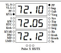
The 7<sup>th</sup> page shows Phase wise KVA for R, Y and B phase.
