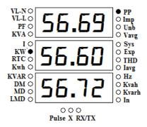
The 5<sup>th</sup> page shows Phase wise KW for R, Y and B phase.
