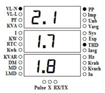
The 33<sup>th</sup> page shows Phase wise Voltage THD for R, Y and B phase. This page indicated by "**VL-N**", "**PP**" and "**THD**"LED glow. In the 3P3W installation "**VL-L**" LED glow instead of the "**VL-N**" LED.
