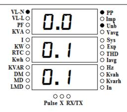
The 35<sup>th</sup> page shows Phase to Neutral/Phase to Phase Voltage unbalance Percentage. Unbalance Percentage is with respect to maximum Voltage. This page indicated by "**VL-N**", "**PP**" and "**Unb**" LED glow. In the 3P3W installation "**VL-L**" LED glow instead of the "**VL-N**" LED.
