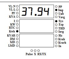
The 10<sup>th</sup> page shows System Import KWh. This page indicated by "**Kwh**", "**Sys**" and "**Imp**" LED glow.
