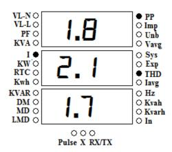
The 34<sup>th</sup> page shows Phase wise Current THD for R, Y and B Phase. This page indicated by **"I**", **"PP**" and **"THD**"LEDs glow.
