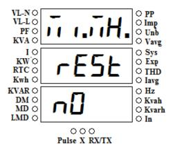
2. Press <sup>(m)</sup> key again. Immediately 'P' starts blinking which shows that the parameter can now be changed. Select "JE5" by pressing ▲ and ▼ keys and then press <sup>(m)</sup> key for resetting Min – Max Data and after the <sup>(m)</sup> Key Press unit automatic reset.
