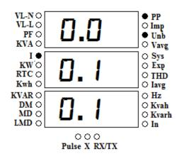
The 36<sup>th</sup> page shows current unbalance Percentage. Unbalance Percentage is with respect to maximum Amps.
