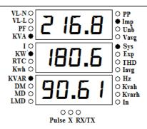
The 8<sup>th</sup> page shows System KVA,KVAR and KW.
