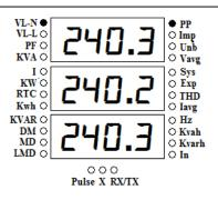
The 2<sup>nd</sup> page shows Phase to Neutral Voltage for R,Y and B phase. This page indicated by "**VL-N**" and "**PP**" LED glow. "**PP**" Stands for Per Phase.
