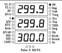
The 3<sup>rd</sup> page shows Phase wise current for R, Y and B phase. This page indicated by "**I**" and "**PP**" LED glow. "**PP**" Stands for Per Phase. This Page will be not available in the 1P2W installation.
