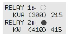
The 30<sup>th</sup> display page shows relay status with its selected parameter for which alarm has to be generated. Value displayed in bracket indicates the value programmed for assigned parameter. Value displayed without bracket indicates run time value of assigned parameter.
