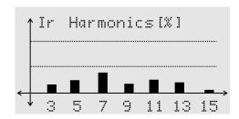
The nineteenth page shows Odd Harmonics Histogram for current in R-phase with percentage form. Likewise, Odd Harmonics Histogram for current in both Y-phase and B-phase will also be shown on 21st and 23rd pages respectively.
